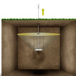
Granular Soil (Based on Terzaghi's calculation)
