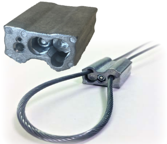
Falcon LockGrip LG-3 provides a two way grip of 1/8" (3mm) wire rope for a variety of bracing applications.
