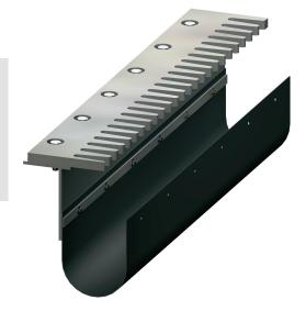
The D.S. Brown Drainage Trough System provides superior performance when trough splices become necessary. For trough splices less than 72 inches, the D.S. Brown Company uses the time-tested and lab-proven method of hot vulcanization to make splices in drainage trough systems. The D.S. Brown Company uses cold-chemical vulcanization for trough splices exceeding 72 inches.
