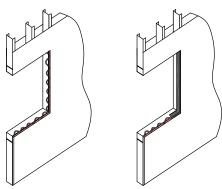
7. Apply a generous bead of AIR-SHIELD LIQUID FLASHING to the vertical surface around the rough opening and spread this material with a W. R. MEADOWS SPREADER TOOL or putty knife in an even, monolithic manner 4" – 6" (100 – 152 mm) onto the vertical surface around the rough opening. Make sure material contains no pinholes and is void-free. Again, make sure material is even, monolithic, and undamaged. Test the thickness to ensure the material has a thickness of 12-15 mils.
