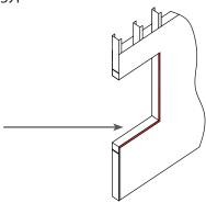
4. Prefill any joints or cracks that are larger than ¼" (6.35 mm) and less than ½" (12.7 mm) with AIR-SHIELD LIQUID FLASHING. Apply a generous bead of material over the joint, press, and spread into the joint. Allow material to skin over prior to full application of AIR-SHIELD LIQUID FLASHING.
