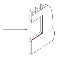
5. Prefill any joints or cracks larger than ½" (12.7 mm) with AIR-SHIELD LIQUID FLASHING. Install KOOL-ROD, into the joint to control sealant depth and apply AIR-SHIELD LIQUID FLASHING. Smooth out using a W. R. MEADOWS SPREADER TOOL or putty knife and allow to cure prior to full application of AIR-SHIELD LIQUID FLASHING.
