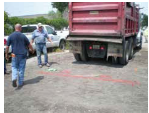
Truck (31 Tons) Backing Over R-Tank LD
