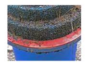
The filter cartridge(s) install through a hole in the bottom of the support deck or collection basin. The hole has four (4) slots that accept 4 tabs molded into the underside of the cartridge body.
