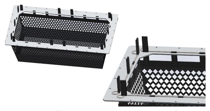
**4.** Using the catch basin frame clear opening length and width measurements from Step 2, adjust the sliding flanges such that they will securely rest on the grate frame. The inside flange to flange distance should be equal to the previously measured clear space for both length and width. Loosen bolts as necessary and adjust sliding drop flanges to the required position and secure in place using a standard 7/16" socket wrench. Do not overtighten bolts.
