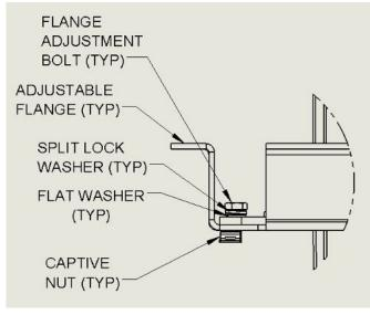
**5.** Carefully lower the StormSack assembly into the storm drain and verify that the support flanges are securely resting on the storm grate support ledges.
