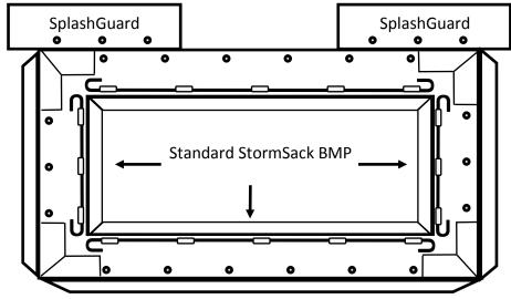
The splashguards are oversized with the intent being to cut them down to fit into the curb throat.
