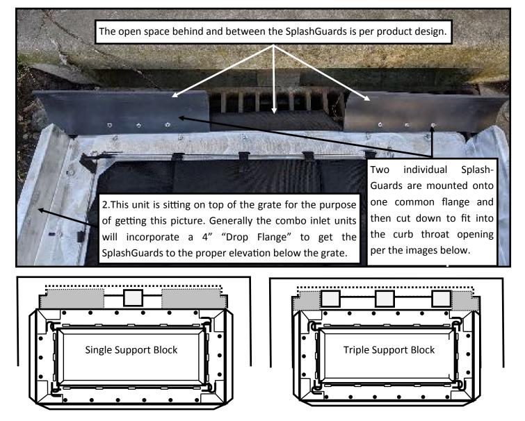
The SplashGuards are cut down to fit the curb throat opening as shown above. Please note that the intent of the SplashGuard is to divert the flow down the curbline into the StormSack BMP unit.
