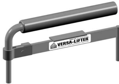
The VERSA-Lifter makes it easier to lift and place units—especially on the base course. Two prongs on the lifter are inserted into pin holes in each Standard unit. Lifting the handle secures the lifter to the unit and makes for easy, balanced lifting and placement.
