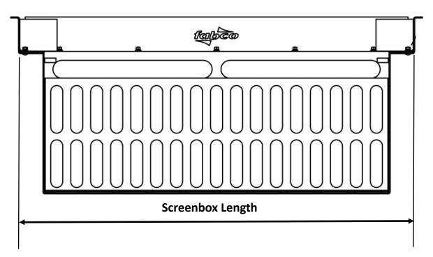
Sliding Flanges should be set at the grate frame clear space measurements
