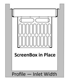
**6.** Corner fillers: ScreenBox units utilize the Fabco adjustable BMP frame/flange system. The adjustability inherently leaves some open space in the corners of the frame. The units will ship with "Corner Fillers" (pictured right) to address the open corner issue. Remove the adhesive tape backing and install the Corner Fillers. For ScreenBox units designed for combination (curb throat) inlets see Step 7 for further
