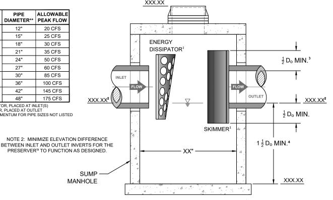
NOTE 3: STOCK SKIMMERS HAVE A MINIMUM FREEBOARD DEPTH OF  $\frac{1}{2}$  D<sub>0</sub>. FOR GREATER FREEBOARD DEPTHS, DESIGNERS CAN UPSIZE THE SKIMMER, OR USE A CUSTOMIZED SKIMMER. FOR CUSTOM DESIGNS, AND/OR PROJECT SPECIFIC DETAILS, CONTACT MOMENTUM.
