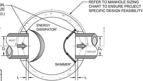
NOTE 1: THE PRESERVER™ ENERGY DISSIPATOR WAS DESIGNED AND TESTED TO FUNCTION WITH OR WITHOUT A SKIMMER. DISSIPATORS & SKIMMERS CAN BE UTILIZED IN TANDEM OR INDEPENDENTLY.
