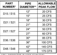
"D" = DISSIPATOR, PLACED AT INLET(S)
