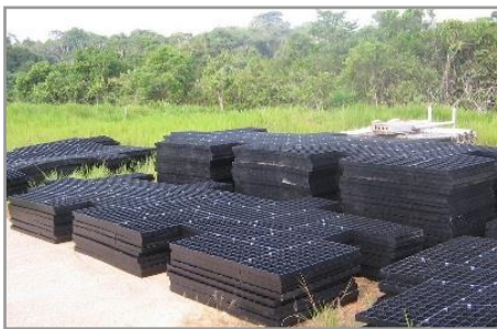
Figure 25: Pre-Assembled GEOTERRA Mats
