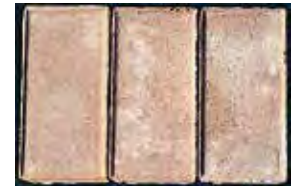
Pavers with efflorescence
