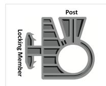
**Figure 1.** ATRA® Tendon Clip Load Transfer Device.
