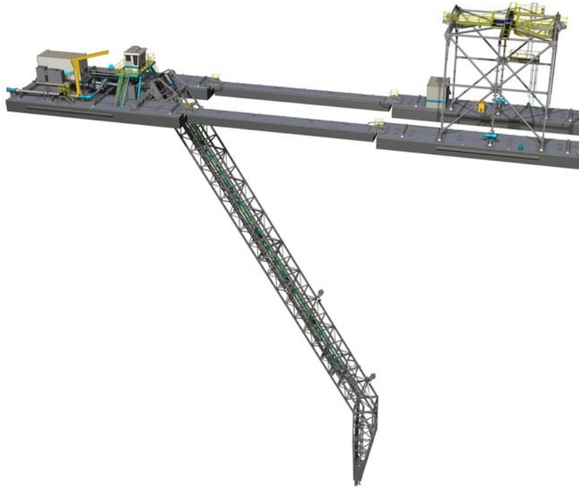
Figure 3. Autodesk Inventor model showing 60 degree down angle.
