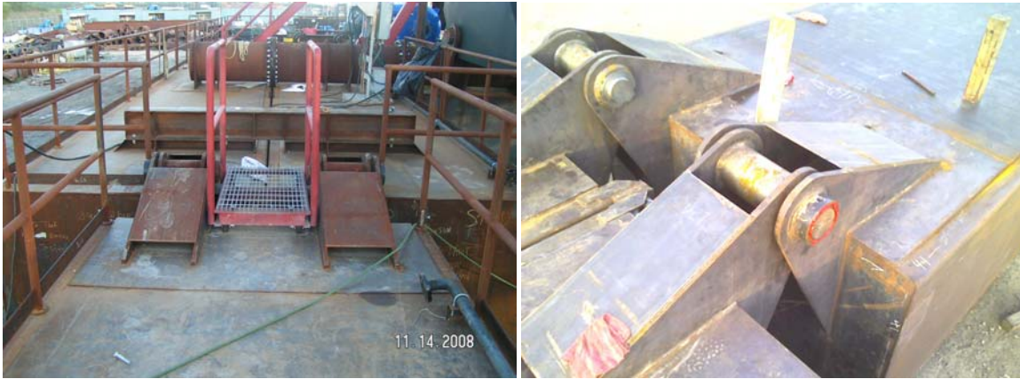
Figure 8. Photos showing hull pin sections that allow for proper trim conditions.
